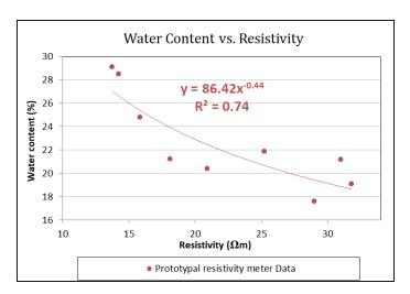
Fig. 3 - Water content relationship with resistivity.
